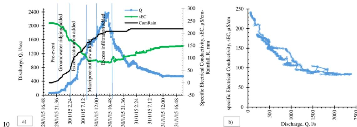
Figure 6. a. Hydro-chemograph plot of the 29-31 January 2015 storm event and related hydro-geomorphological phases, during which the runoff components are progressively added, according to Table 3; b. Q-EC hysteric cycle of the storm event.
