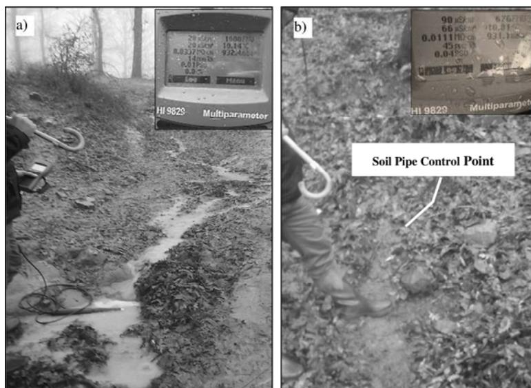
10 Figure 5. Measurements at 12:00 am in the dirty road point controls (a) and the soil pipe (b) with respective sEC measurements.
